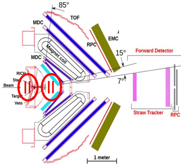
Low Gain Avalanche Detectros for the HADES reaction time (T<sub>0</sub>) detector upgrade:
