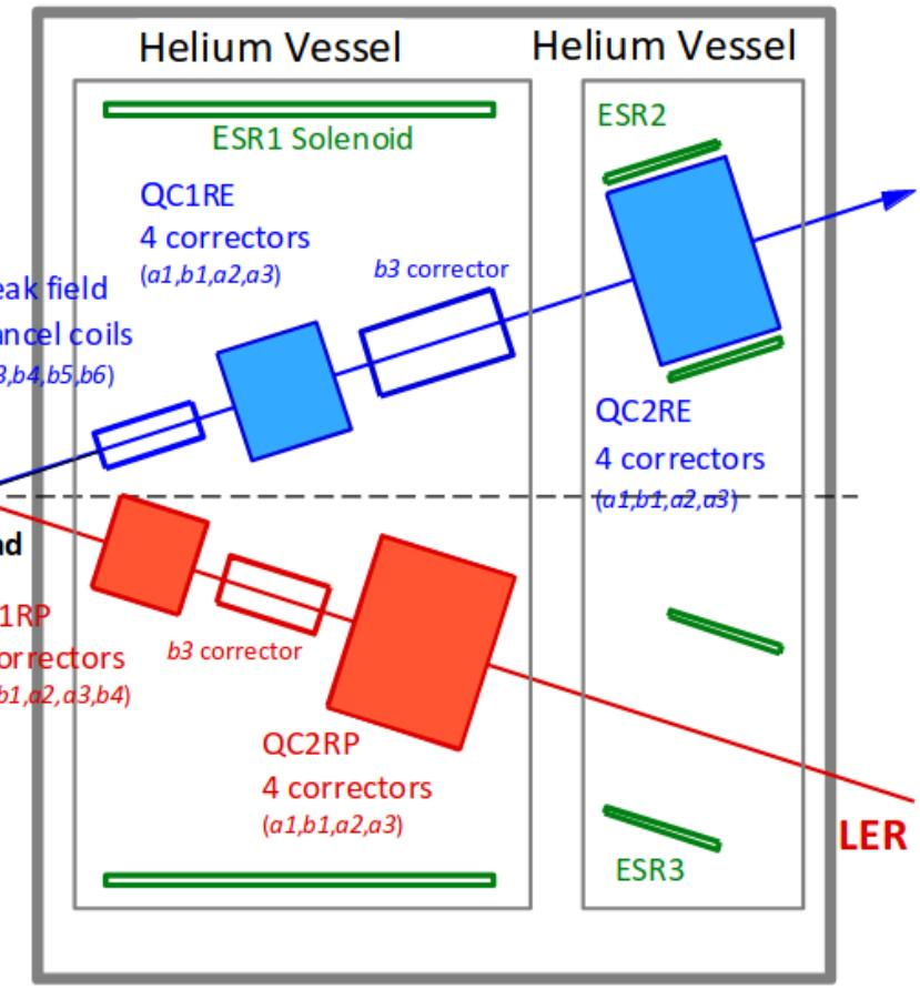
4 SC main quadrupole magnets: 1 collared magnet, 3 yoked magnets
