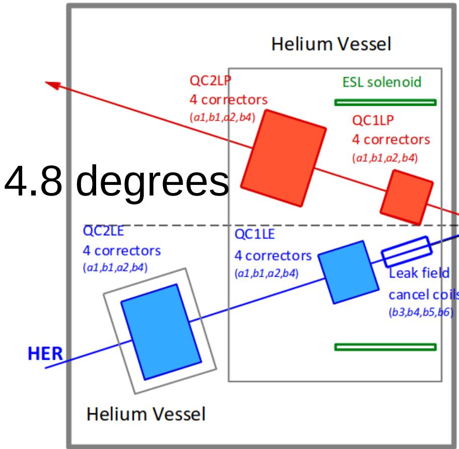
4 SC main quadrupole magnets: 1 collared magnet, 3 yoked magnets
