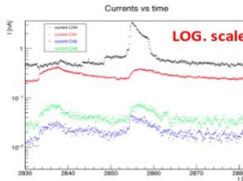
Ionizing current seen by diamond sensors at various locations during vacuum scrubbing
