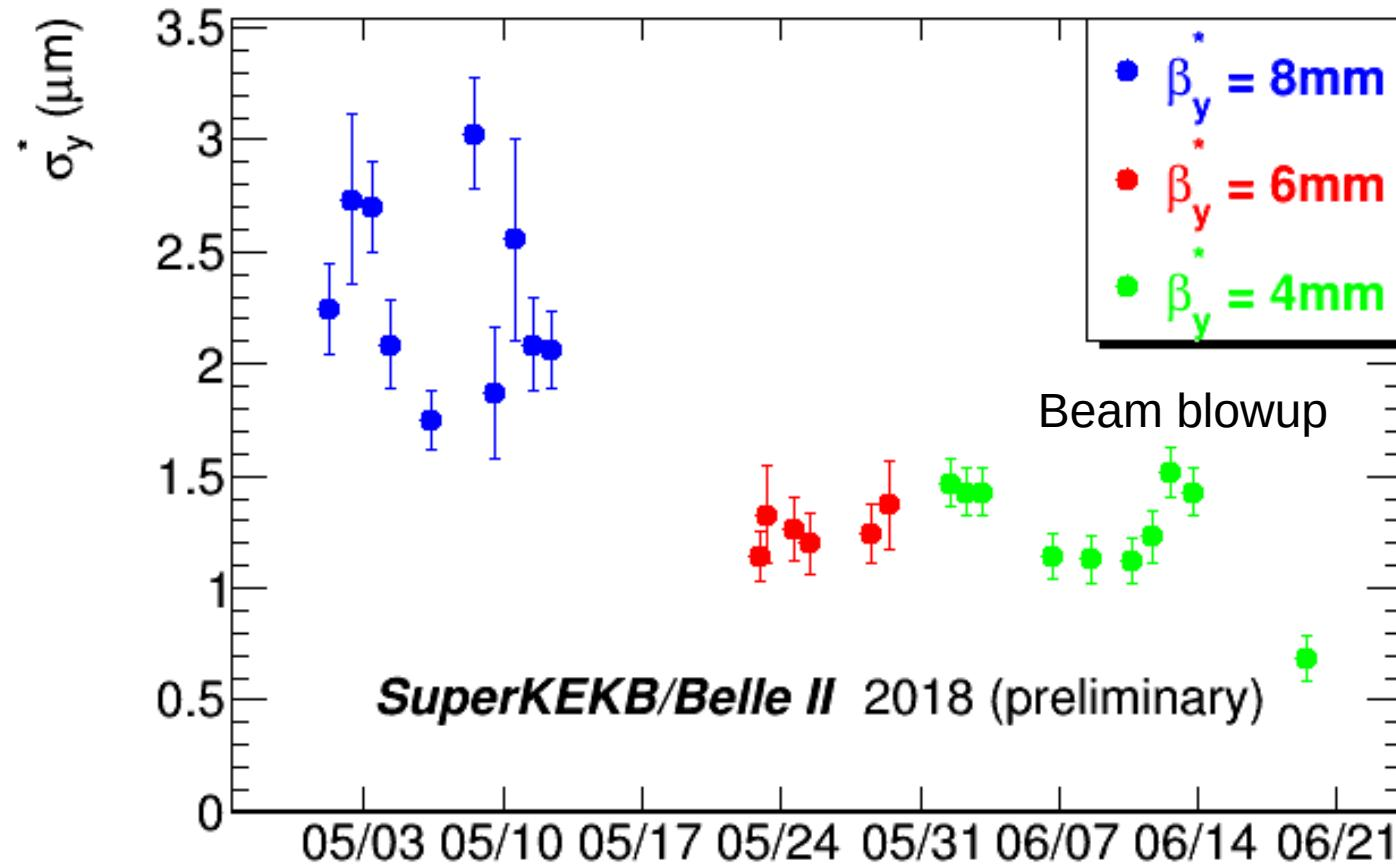
At Phase 2 peak luminosity the vertical spot is  $\sim 700 \text{ nm}$  high. There is still beam-beam blowup at high currents. At low currents, the vertical spot size is  $330 \text{ nm}$  high (the final goal is  $\mathcal{O}(50\text{nm})$  with full capability of the QCS system).
