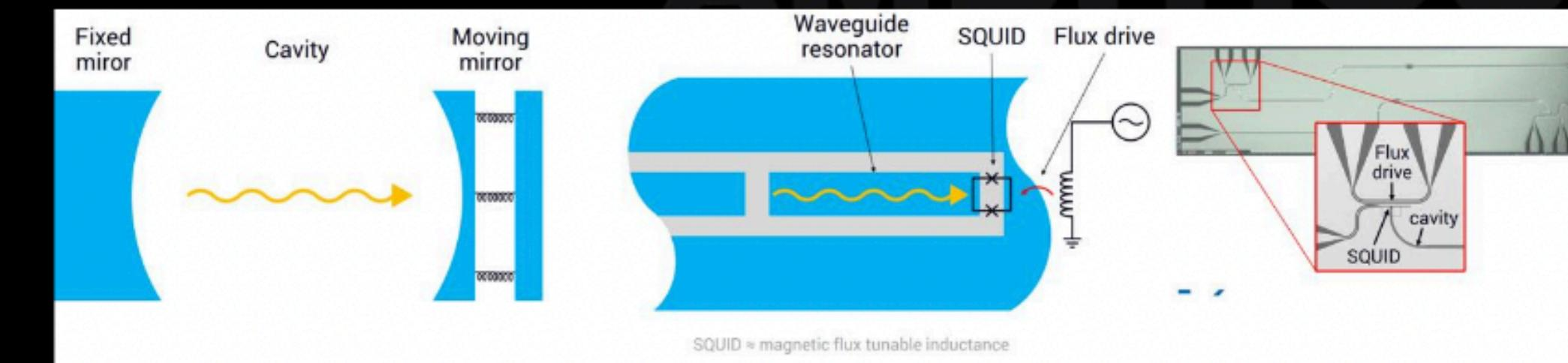
Figure 2: Cavity resonant setup (images from FBK)
