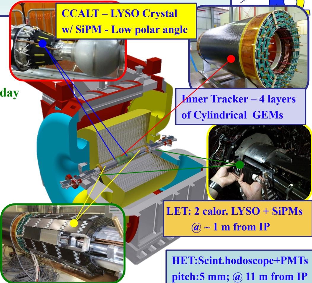
**QCALT – Tungsten / Scintillating Tiles w/ SiPM Quadrupole Instrumentation**
