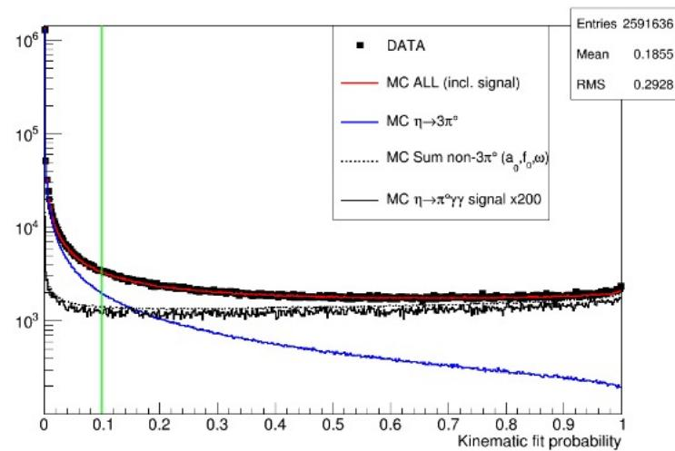
4. **Kinematic fit with 11 constraints (9 + mass of  $\eta$  and  $\pi^0$ ) to reject  $\phi \rightarrow a_0(980)\gamma \rightarrow \eta\pi^0\gamma$  events  $P(\chi^2) < 10\%$**
