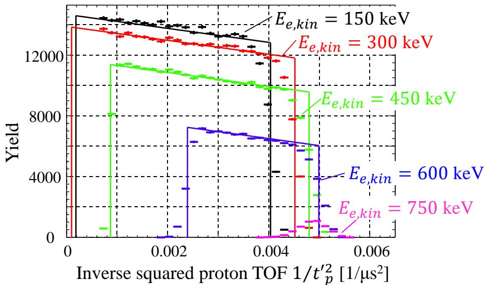
Data analysis: Use **edge** to determine or verify the spectrometer TOF response function.
