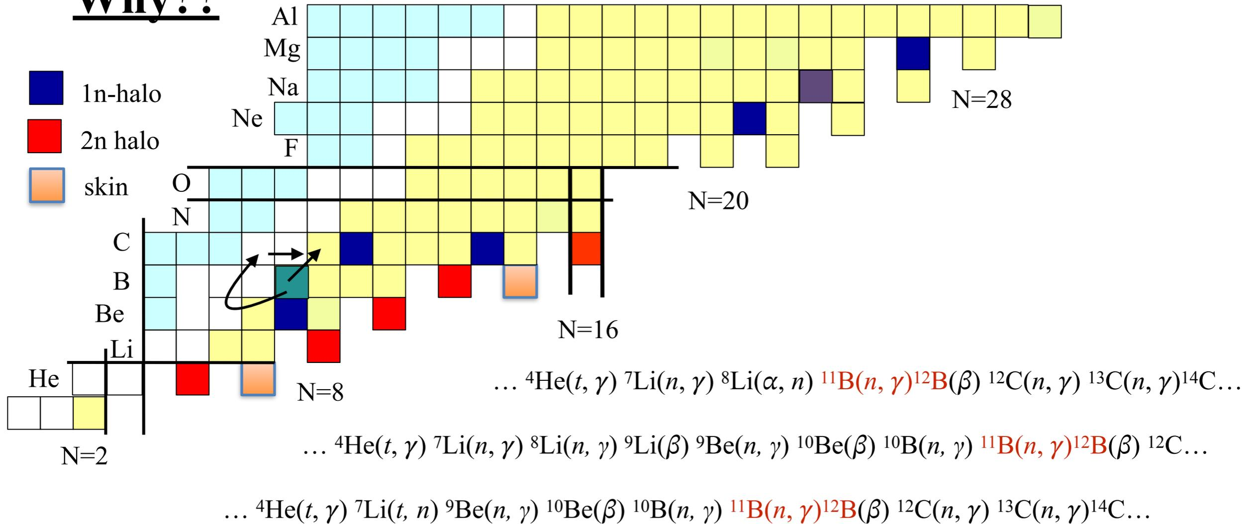
The  ${}^{11}\text{B}(n, \gamma) {}^{12}\text{B}$  reaction is vital to all these chains...
