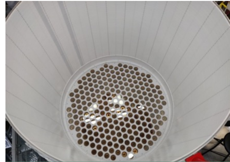
494 TPC PMTs (Hamamatsu R11410-22) Photo: bottom array + field cage
