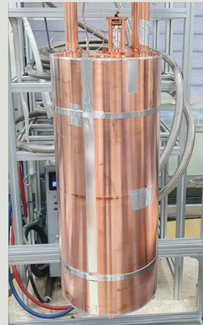
Resonant Cavity Copper tuning rod ID 272 mm, Q_0 \sim 100,000
