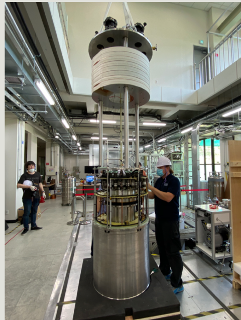
Superconducting magnet Center field 12 T @ 4.2 K Bore diameter of 320 mm
