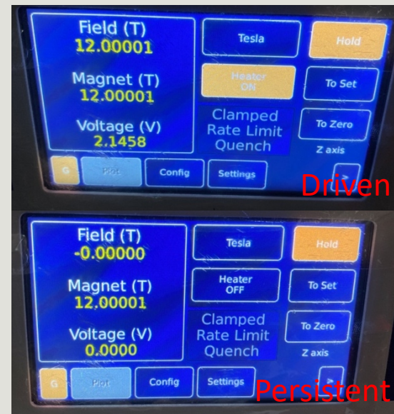
12 T shown in Magnet (T) for both driven (top) and persistent (bottom) mode
