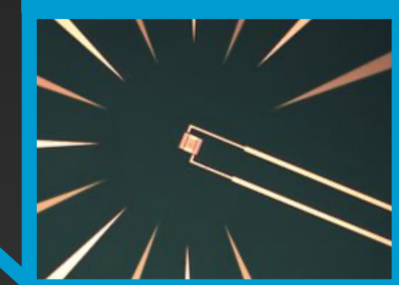
TES: Tungsten microchip operating at T_C \sim 140 mK from NIST ( 25 \mu\text{m} \times 25 \mu\text{m} )
