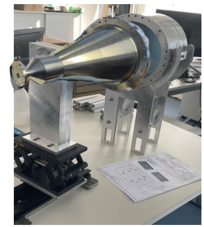
CB200 Closed booster Cu mirror ≥3 Ø200 mm discs
