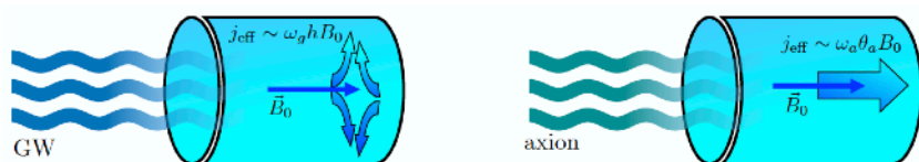
FIG. 1. A cartoon illustrating the differences between GW-EM conversion (left) and axion-EM conversion (right) in the presence of an external magnetic field \mathbf{B}_0 . The GW effective current is proportional to \omega_g h B_0 , with a direction dependent on the GW polarization and a typical quadrupole pattern, yielding a signal field with amplitude h B_0 . The axion effective current is proportional to \omega_a \theta_a B_0 , with a direction parallel to the external field \mathbf{B}_0 , yielding a signal field with amplitude \theta_a B_0 . The differing geometry of the effective current yields different selection rules for coupling the GW and axion to cavity modes.
