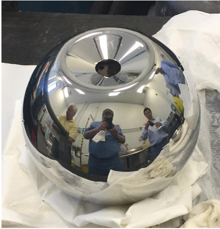
Inverted Gun Cathode Shroud
