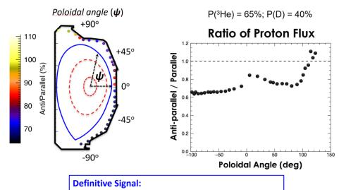
lpha and p loss-locations on the Tokamak wall depend upon the initial polarizations.
