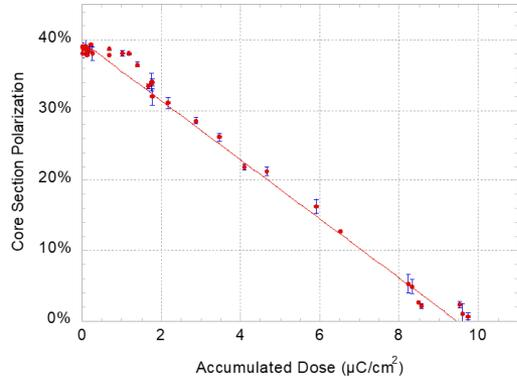
Run 3B: Core Polarization VS Core Dose/Area
