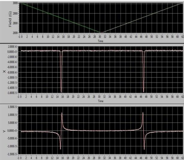
Proton Signal from PD, ~40% Polarization
