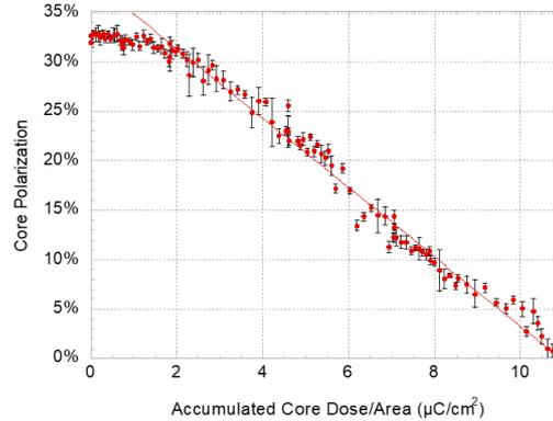
Target polarization lost (almost) linearly as Areal Dose accumulated.
