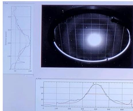
Rastered beam profile on a YAG
