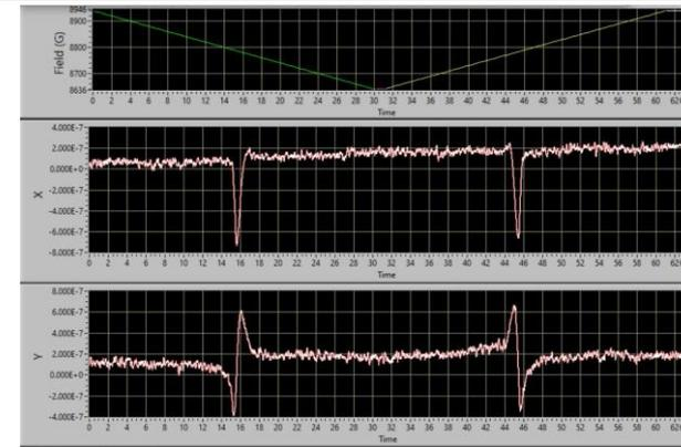
Proton Signal from IBC, ~40% Polarization,
