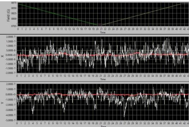
Typical TE Signal from IBC, 170 scans,  $I_e = 0$  pA
