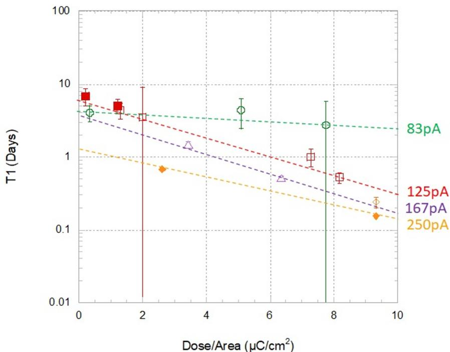
Runs 3A and 3B: Relaxation Times VS Average Beam Current at an Accumulated Core Dose/Area =  $5.0 \mu\text{C}/\text{cm}^2$
