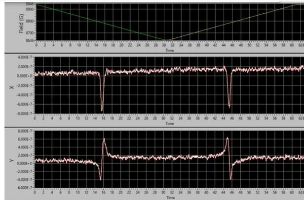
Proton Signal from IBC, ~40% Polarization,
