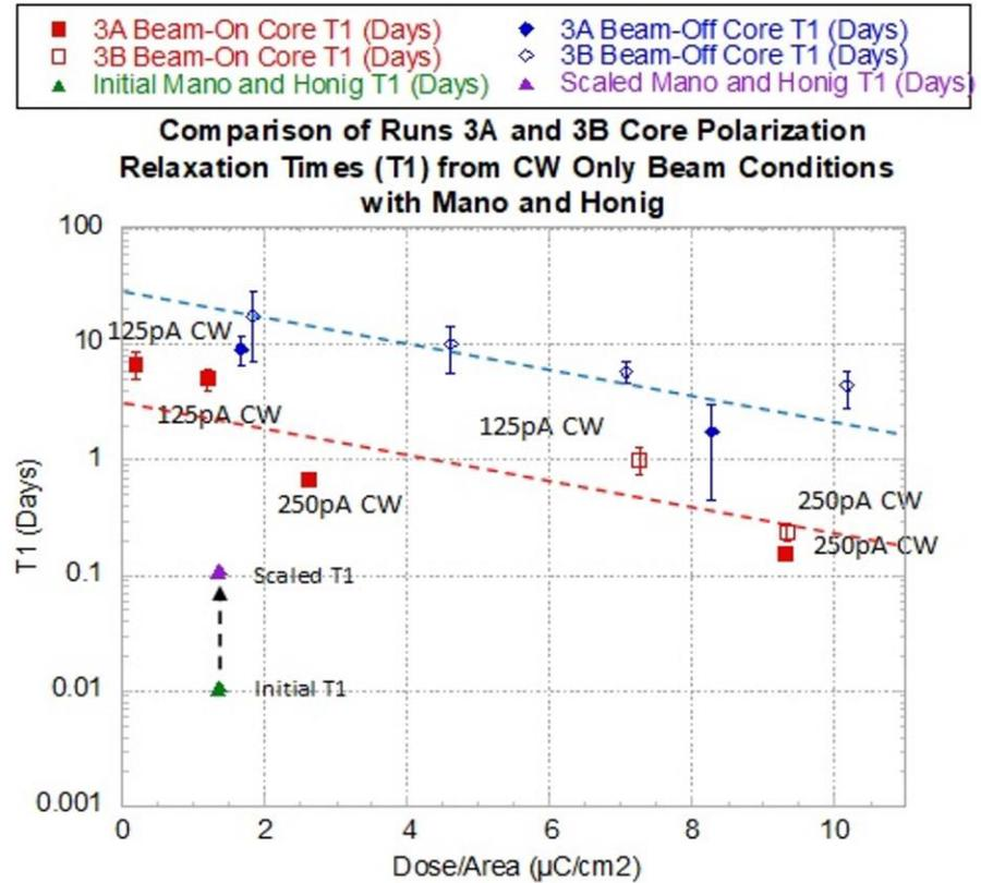
The same model used to scale Mano and Honig's  $T_1$  values can be used to project the relaxation times for ideal conditions.
