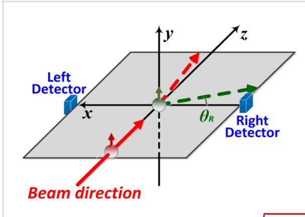
The beam ( $\uparrow\downarrow$ ) and target ( $\pm$ ) single spin asymmetries are concurrently measured in the  $0.5 < T_R < 10$  MeV recoil energy range.
