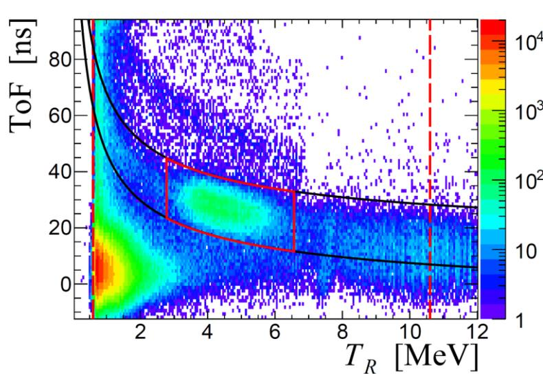
To isolate elastic  $pp$  events, the measured recoil proton energy is compared with the time of flight
