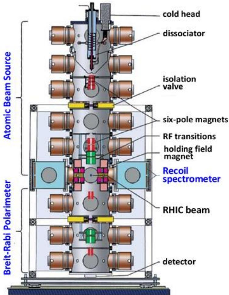
Since 2004, the HJET is used to measure the absolute proton beam polarization at RHIC
