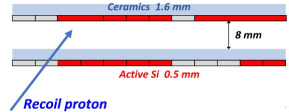
The goal was to veto punch-through  $\pi, p, d, \alpha, \dots$ , which are expected to have momentums of 100-500 GeV/c. The ceramics between layers must not be the problem for that.
