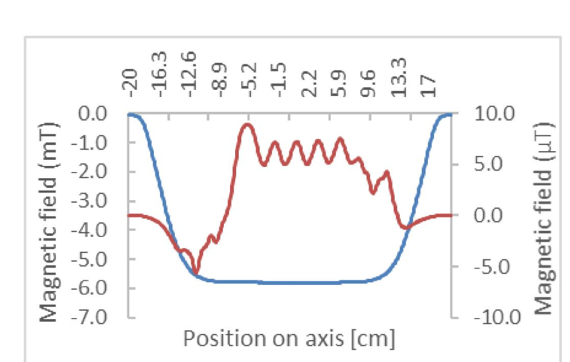
• **SIMULATIONS:** It is preponderant to minimize the impact of the magnetic field induced by the permanent ring-magnets added in the modifications, to the one produced by the coils at the beam path
