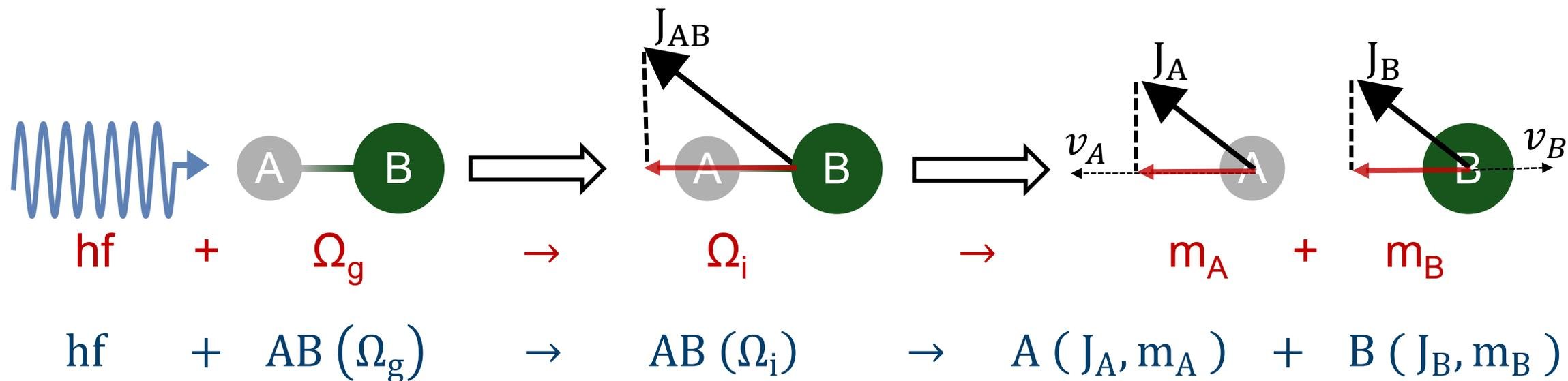
$\Omega_i$  is the **projection** of the total electronic angular momentum of electronic state  $i$  along the AB bond axis.
