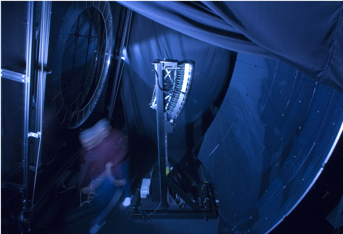
Schmidt telescope: corrector ring, 440 PMT camera, mirror
